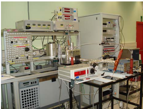
Fig. 1 Photograph of the new INTA high-range standard humidity generator
